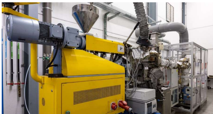
Certech digitized pilot line for pyrolysis of waste plastics, comprising a single screw extruder (left) feeding plastic waste in continuous mode to a 20 L reactor with a collection station (right), encased within a transparent protective enclosure. Copyright@ Certech 2024.
