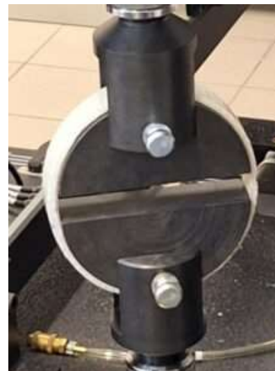
Accessory developed by Certech for the determination of the tensile strength of thermoset polymer pipes (ISO 8521:2020 standard) - Copyright@ Certech 2024
